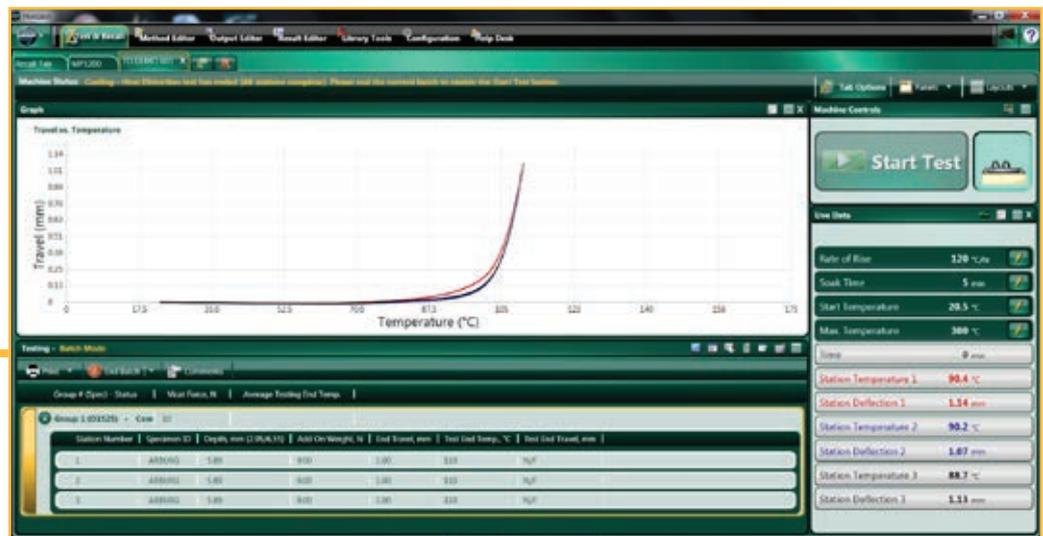
**Results** from a six station Deflection Temperature Under Load test run on an HDTM603.
